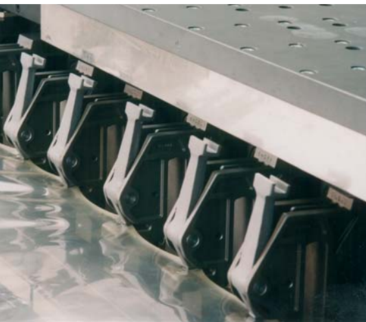
LISIM clips picking up PET film. The temperatures of individual clip rolls and bearings are constantly monitored to prevent damage.
