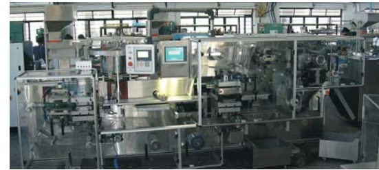
The rotary cutting station and blister pickup assembly can be seen on the right side of the image. They are driven by the servo motor and synchronized with the speed of the foil. This pickup assembly drops the blister pack at 45 degrees if the blister contains empty tablets or at 90 degrees if it is OK.
