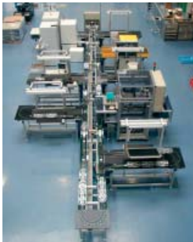
Production line for antenna amplifiers.
