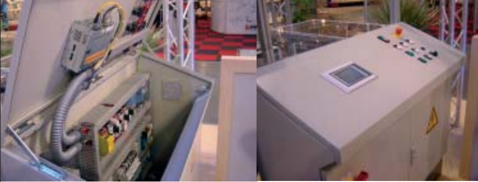
Switching cabinet view: Using the PP200 Power Panel for the complete control and visualization of the production line.
