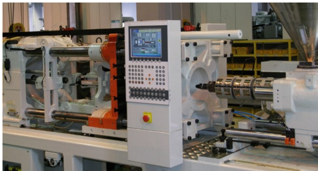
Injection and clamping unit on a Dongshin (Korea) injection molding machine, featuring a B&R automation solution.
