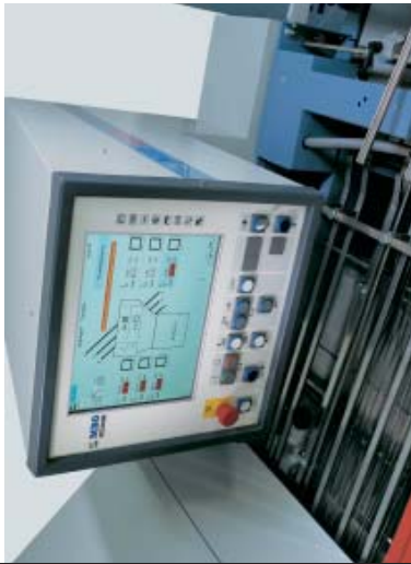
The MBO Navigator-Control machine controller is a modern digital microprocessor controller which combines machine control, product monitoring, and the machine configuration into a single control management system.
