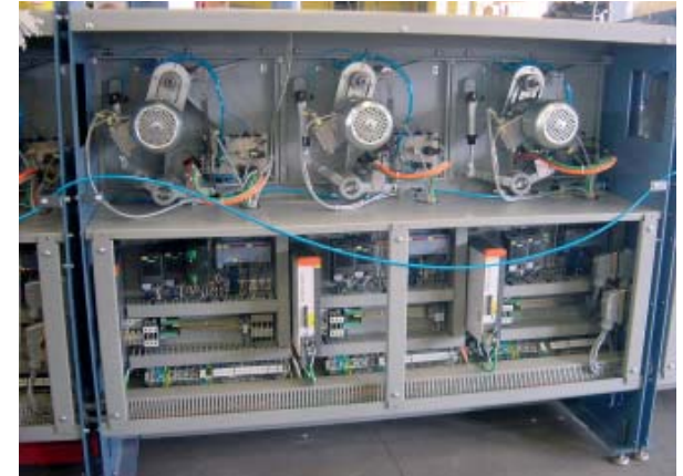
DS10 switching cabinet. One ACOPOS unit is used per spool drive as the spindle drive.
