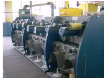
A look at the „brains“ of the 10-headed DS10 from Dietze+Schell. A Provit 2000 Industrial PC controls up to twelve ACOPOS servo axes for rewinding synthetic and spun yarn.
