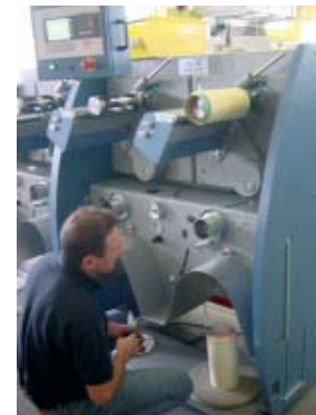
Commissioning of the 8-headed DS10 crosswound bobbin machine with electronic laying system (ACOPOS) for winding speeds up to 1,200 meters/min.
