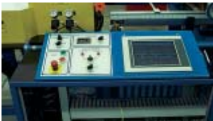
A control station, used to monitor and change all machine settings of the pouch machine.
