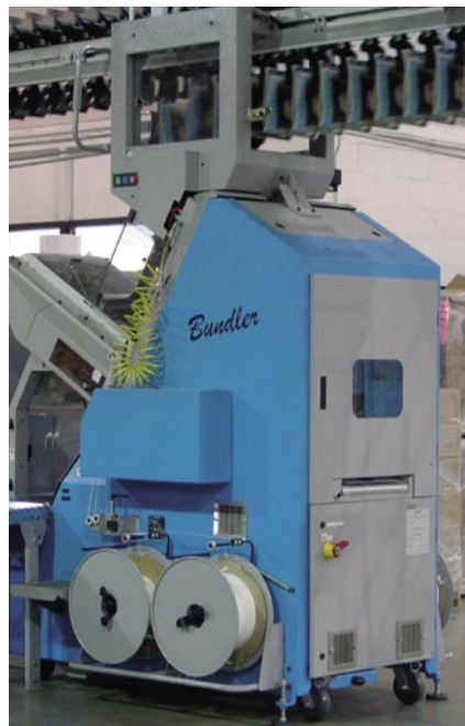
GMA's bundler is presently able to output 1,500 bundles per hour.
