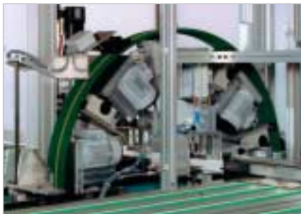
The rotating ring mechanism with processing tools is the heart of the new machine generation
