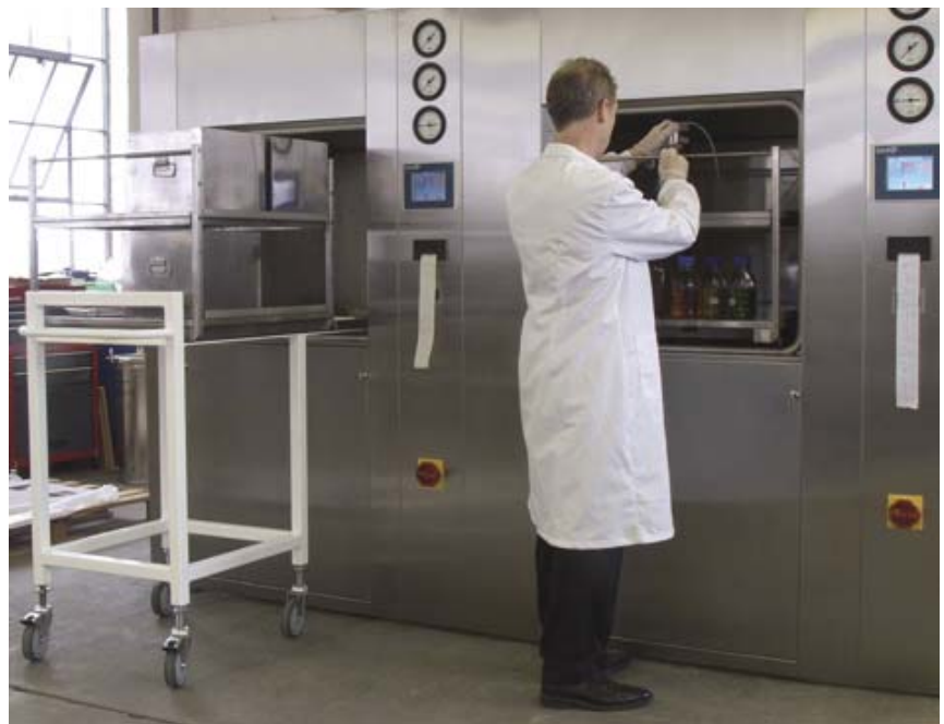
Astell autoclaves with rectangular section. In the non-sterile outside area the load is placed into the opening and the sterilization process is started.
