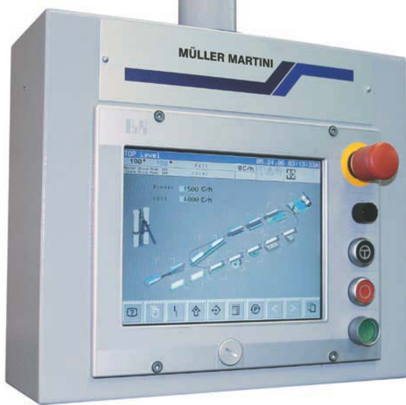
The customized Power Panel allows Muller Martini to create an optimal control, operation and visualization for the Pantera.
