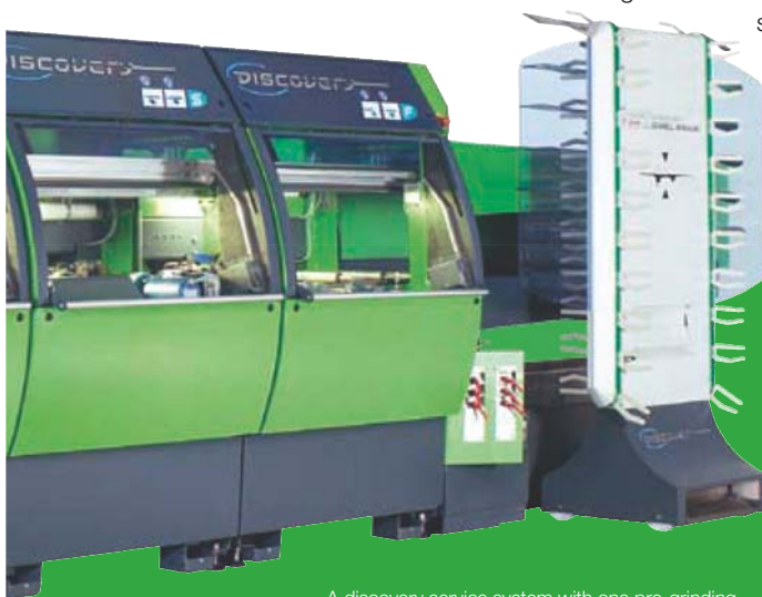
A discovery service system with one pre-grinding-, two stone/disc-, one finish module and two automatic conveyer magazines.
