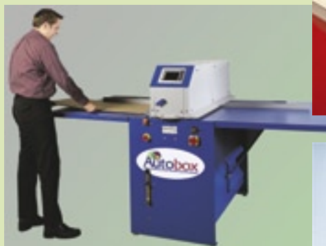
The intuitive operator interface employs a Power Panel with Touch Screen. Box style, size, operating speed and many other parameters are set using clear, easy to understand graphics and symbols. Even multiple interface languages are no problem.
