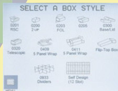
The intuitive operator interface employs a Power Panel with Touch Screen. Box style, size, operating speed and many other parameters are set using clear, easy to understand graphics and symbols. Even multiple interface languages are no problem.
